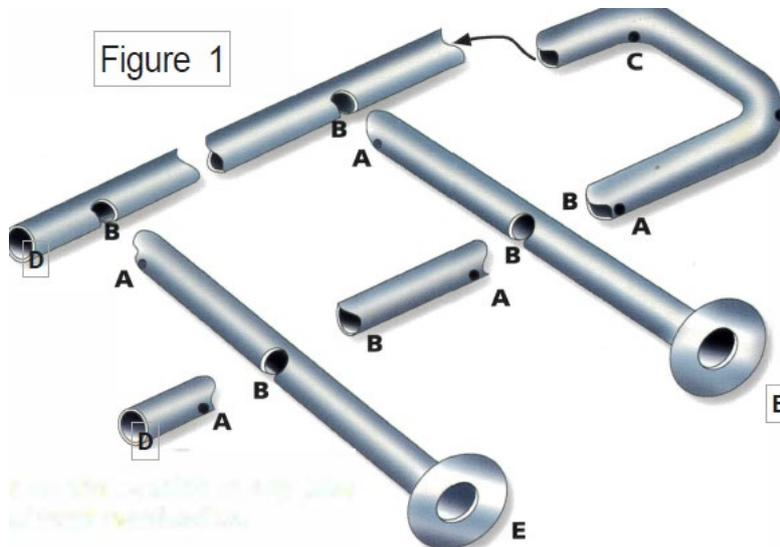
**Vent holes should be visible on the outside of any pipe assembly to provide internal vent verification.**
