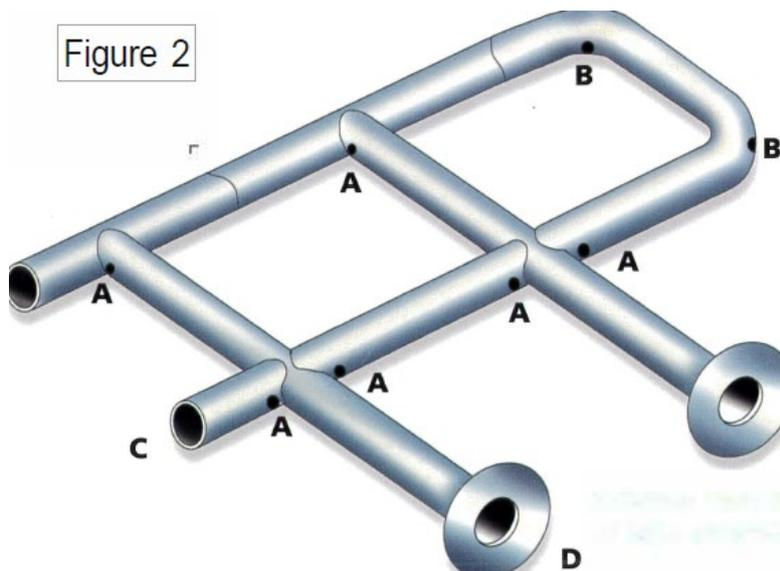
A. Each external vent must be as close to the welds as possible and must be 25% of the I.D. of the pipe but not less than 3/8" (9.5 mm) in diameter. The two holes at each end and at each intersection must be 180° apart and in the proper location.
